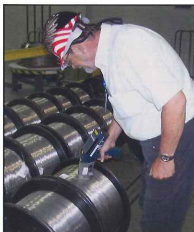
Rigorous positive material identification checks are built into every product.
