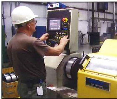
The BIMA Precision Winder produces high-quality layer wound welding spools.
